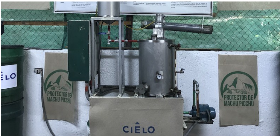
Almost inconspicuous but so important: the biodiesel plant at Inkaterra Machu Picchu Pueblo Hotel © Hanna | Green Pearls®
